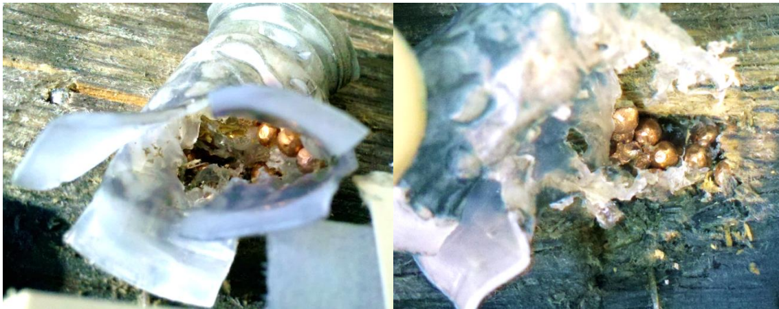
Figure 9: Stuck shot lump in the cup and the wood panel after shooting with FOB Sweet Copper (from Fäth et al. 2018b).
