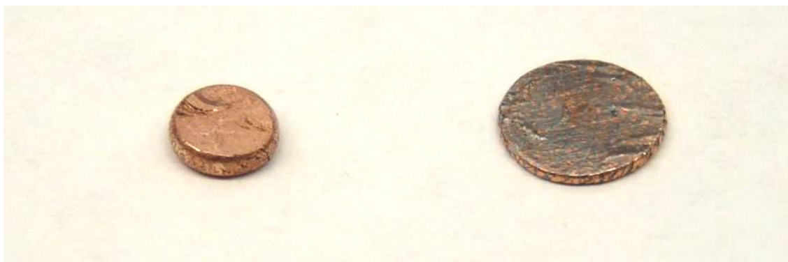
Figure 12: Shot of the FOB Sweet Copper cartridge (declared as lead-free) after a compression test; left: copper shot; right: copper-coated lead shot (from Fäth et al. 2018a).
